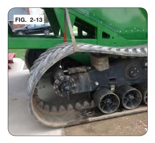
7. Remove the idler hubs (FIG. 2-14).
