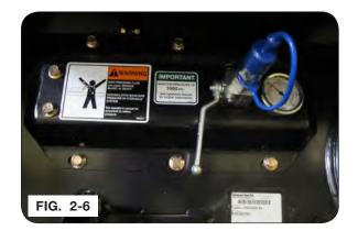
NOTE: If system does not hold pressure, it is possible that there is air in the lines. Follow steps 1-3 but leave the track valve open and cycle the hydraulics on the tractor from extend to float. Engage the hydraulics long enough to completely tension the track then switch it to float and allow the track to detension. Follow these steps 3 to 4 times then retension to 1000 psi and shut the track valve.
