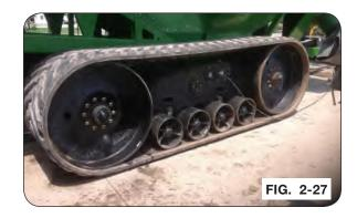
Remove the four bolts and retainer plate that attaches the track assembly to the cart. Retain the bolts and plate for later use (FIG. 2-28).
