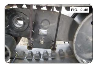
14. Loosen hardware fastening bogie pivot pin to the track. First, remove the roll pin on the slotted hex nut. Next, remove the slotted hex nut and finally remove the bolt holding the teardrop. Once removed, the bogie pivot pin can be discarded.
