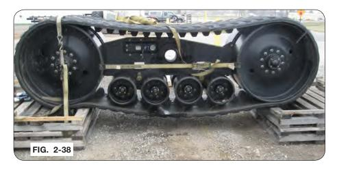
Hook hydraulic tensioner hose (268345) to tractor and place tractor hydraulic lever in float position. Open valve to relieve belt tension pressure and drop pressure down to zero PSI. Allow track to de-tension for 5 minutes.
