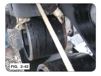
11. Remove the (4) spindle retainer bolts and hardware. Retain for use during reassembly.
